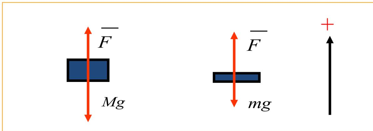
$$I_1 = (\bar{F} - mg) \Delta t = -mv - (-m \sqrt{2gh})$$
