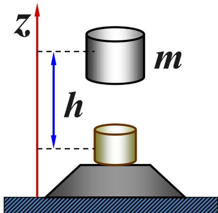
$$\int_0^{\Delta t} (N - mg) dt = m v_z - m v_0 = m \sqrt{2gh}$$
