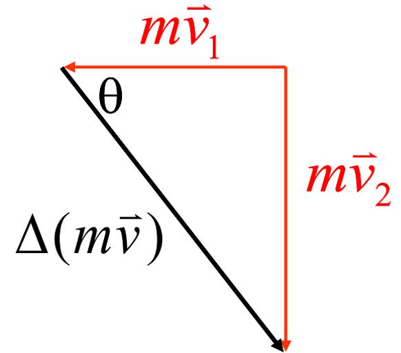
$$|\Delta m\vec{v}| = \sqrt{(mv_1)^2 + (mv_2)^2} = \sqrt{2\pi^2 + 4\pi^2} = \sqrt{6}\pi \quad (\text{kg} \cdot \text{m} \cdot \text{s}^{-1})$$
